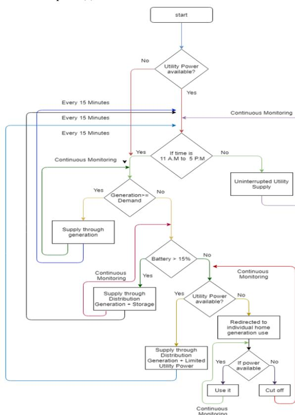
Fig. 5. Street electricity supply algorithm
