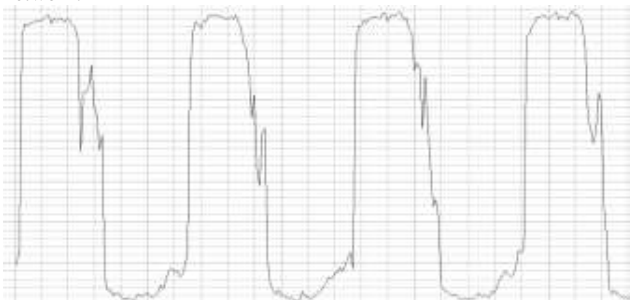
Figure 4 Measured voltage values using Raspberry Pi after separation of common network points
