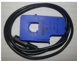
Figure 5. Current clamp meter YHDC SCT 013-20 (current transformer)
