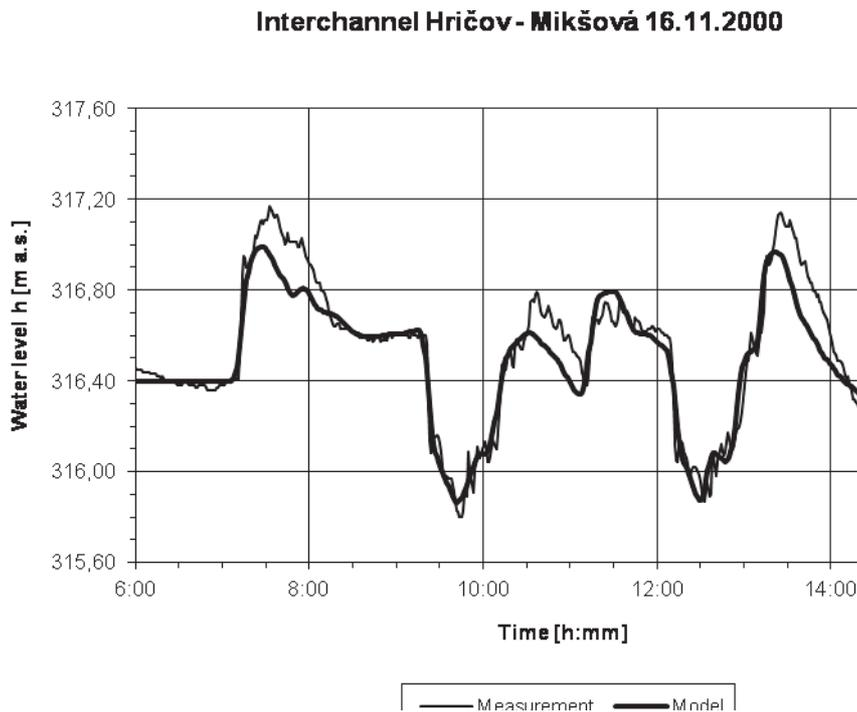
Fig. 3 Comparing water level measurements to results from model
