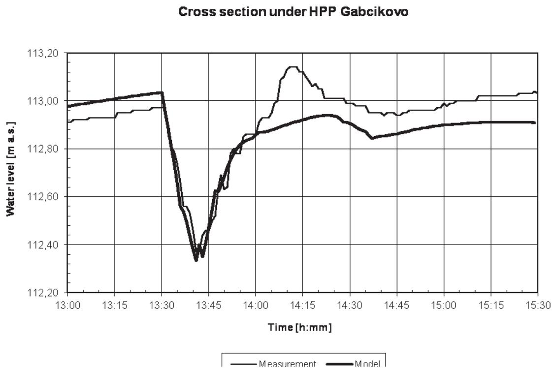
Fig. 8 Comparing water level measurements to results from model
