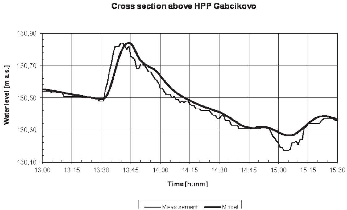
Fig. 7 Comparing water level measurements to results from model
