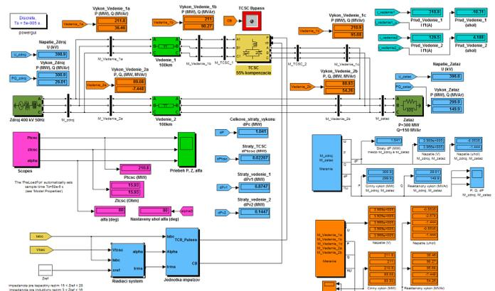
Figure 6. Model of electrical network with TCSC at adjusted angle  $\alpha = 80^\circ$
