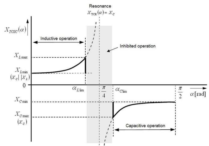
Figure 2. Operating diagram of TCSC [2]
