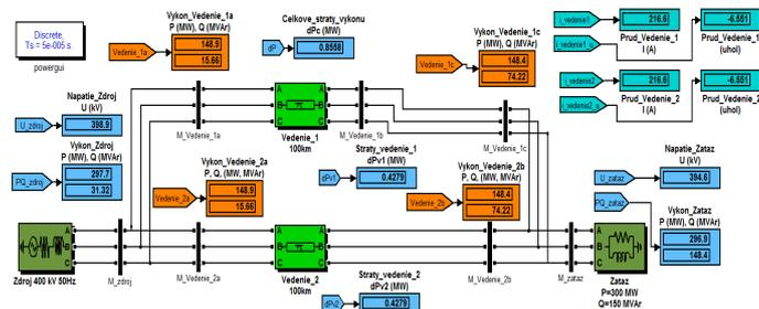
Figure 5. Model of electrical network without TCSC
