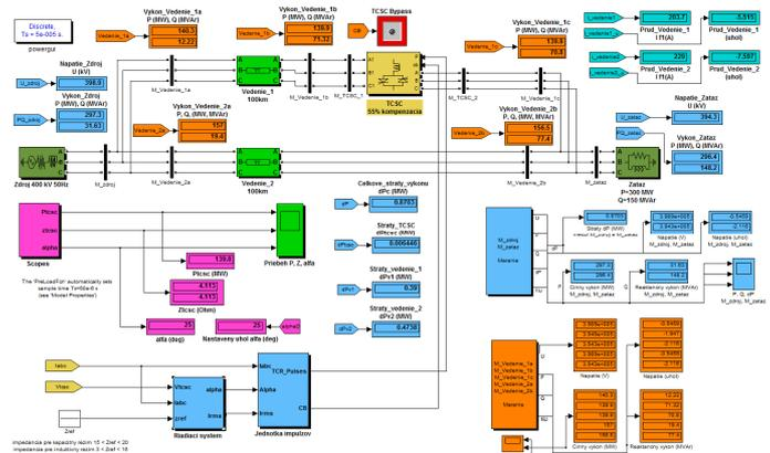
Figure 7. Model of electrical network with TCSC at adjusted angle  $\alpha = 25^\circ$
