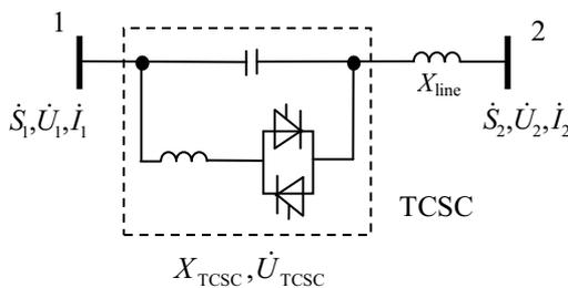
Figure 3 Diagram of transmission path with TCSC
