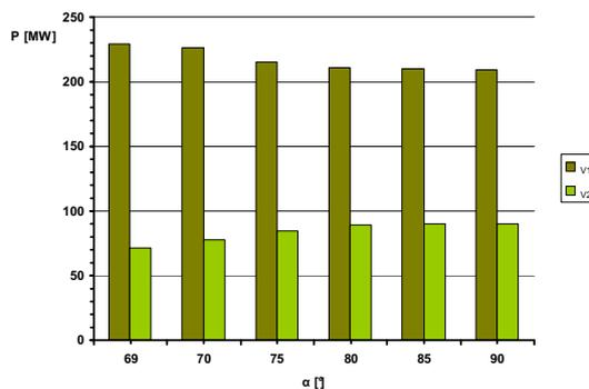
Figure 9. Variation of power flows through lines with angle  $\alpha$  at capacitive operation of TCSC
