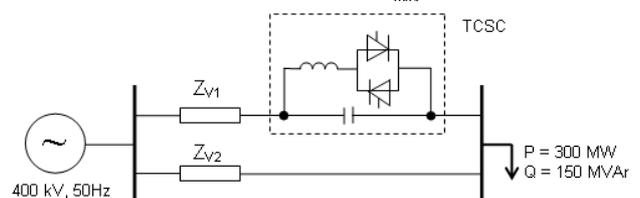
Figure 4. Block diagram of the model of electrical network with TCSC
