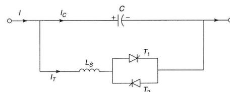
Figure 1 Basic diagram of TCSC
