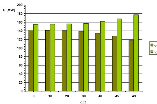
Figure 8. Variation of power flows through lines with angle  $\alpha$  at inductive operation of TCSC
