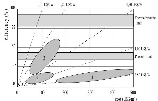
Fig. 2 Efficiency and cost relations of three generations of photovoltaics
