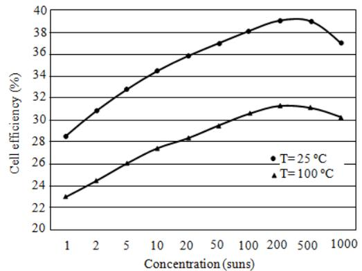
Fig. 4 The efficiency evolution versus concentration ratio at two different temperatures
