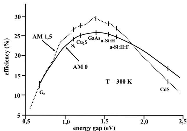
Fig. 3 Dependencies efficiency of respective solar cells on semiconductor energy gap
