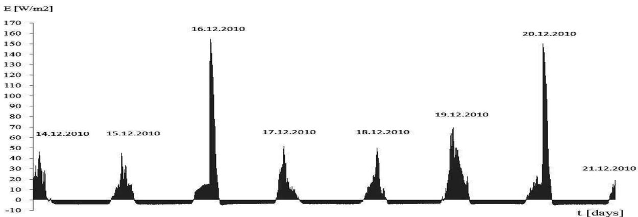
Fig. 2 One-week recording of solar radiation at SUT FEEIT Bratislava
