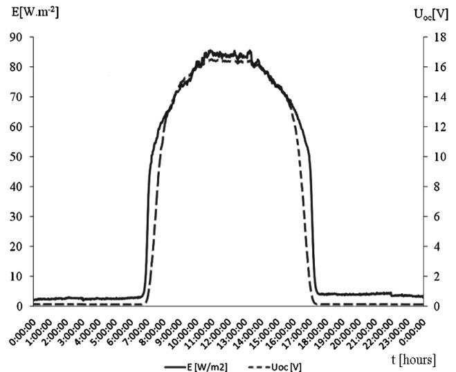
Fig. 3 One - day compare of measured intensity of solar radiation and open circuit voltage on PV structure
