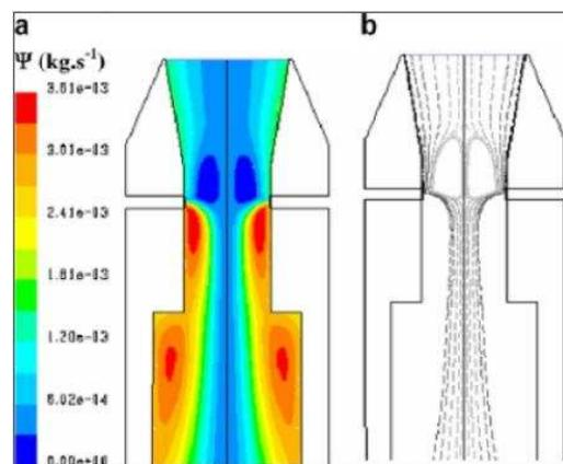
Figure 9. Stream function and gas pathlines in the reactor.
