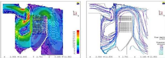
Figure 10. Gas velocity contours and trajectories in a tube bank.
