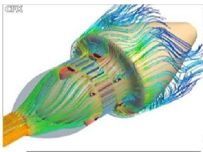
Figure 6. Airflow around generator of wind turbine.
