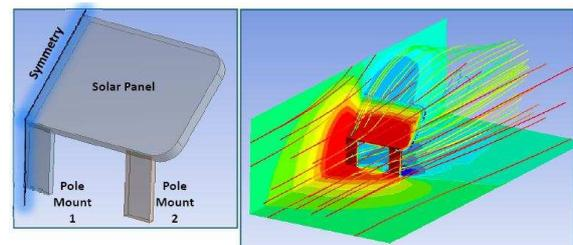
Figure 2. Geometry of the model and ANSYS analysis.
