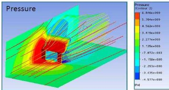
Figure 4. Pressure contour plot.
