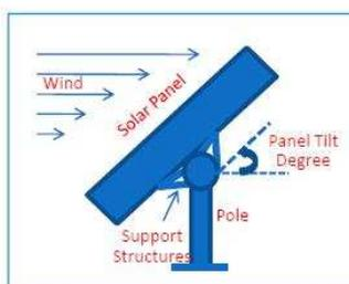
Figure 1. Model of solar panel.
