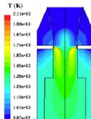
Figure 8. Temperature profile in CFD model of reactor.
