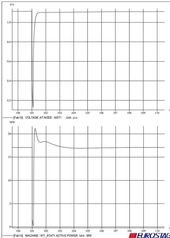
Figure 4. The evolution of the voltage at node NST1 and the active power produced by the WT\_STAT1.
