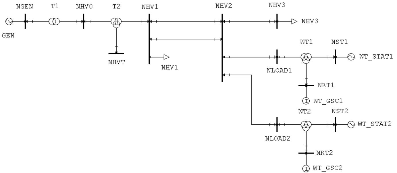
Figure 3. Scheme of modelled electric power system.
