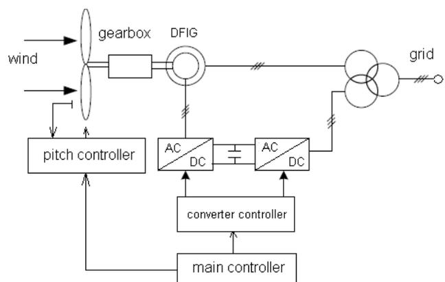
Figure 1. Control scheme of DFIG-based wind power plant.
