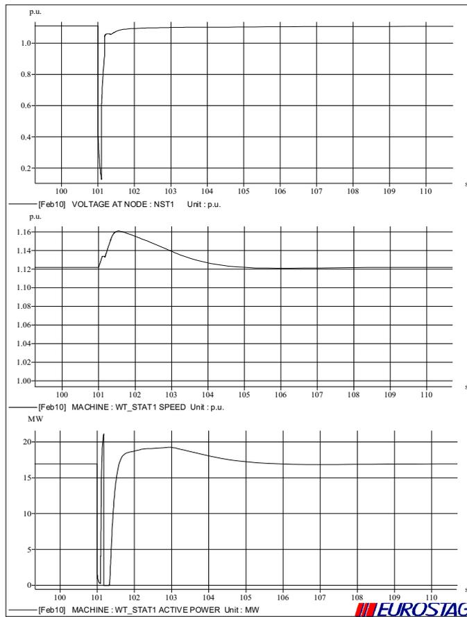
Figure 6. The evolution of the voltage at node NST1, the speed of the machine WT\_STAT1 and the active power produced by the WT\_STAT1.
