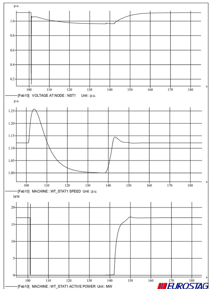
Figure 5. The evolution of the voltage at node NST1, the speed of the machine WT\_STAT1 and the active power produced by the WT\_STAT1.
