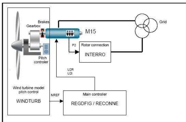
Figure 2. Macroblocks connection of the DFIG model.
