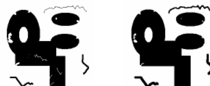
Fig. 6. An example of dilation operator by 3x3 structuring element
