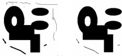
Fig. 7. An example of erosion operator by 3x3 structuring element
