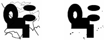
Fig. 8. An example of opening operator by 3x3 structuring element
