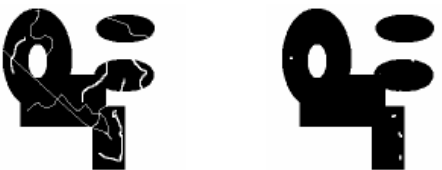
Fig. 9. An example of closing operator by 3x3 structuring element
