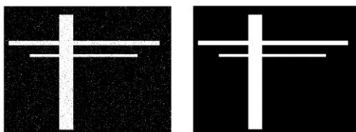
Fig. 2. 2D binary image with dot noise (left) and morphologically filtered result (right)
