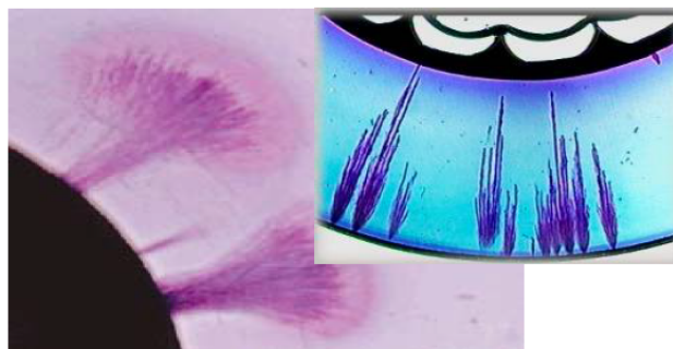
Fig. 2 Water trees growing from the inner (bottom) and outer (top) semiconductive screens [14]
