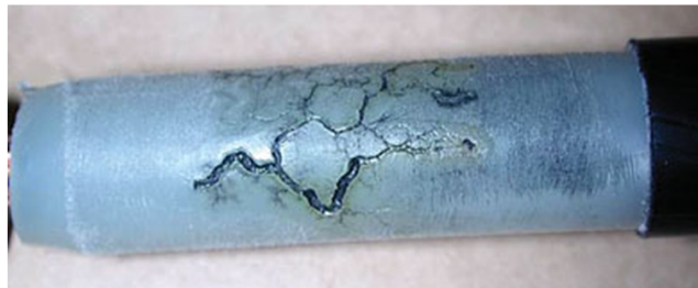
Fig. 1 Damage of XLPE insulation due to ageing
